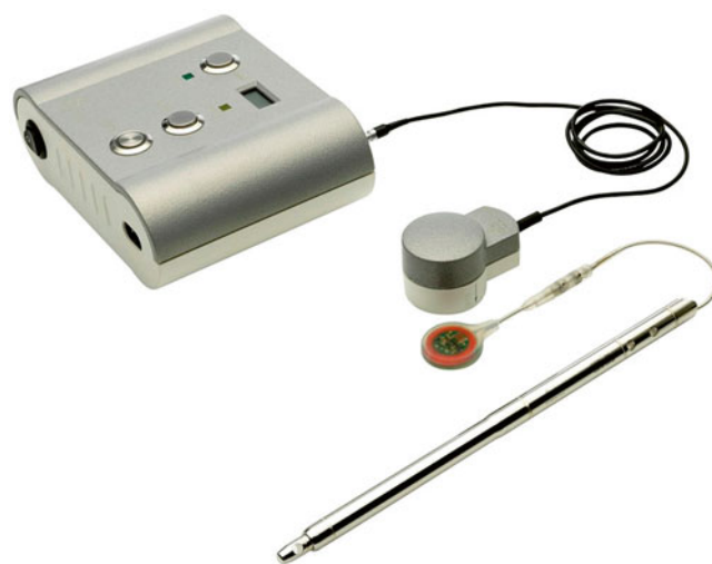
Fig. 9.3 The FITONE nail has an attached cable and antenna. The transformer box shown converts electric current to radiofrequency waves, transmitting energy transcutaneously
